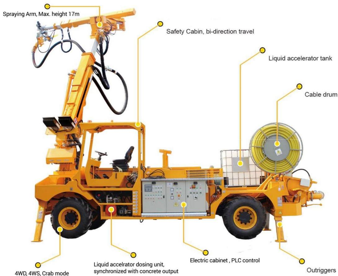
The Atlantic RSA 500 Shotcrete Spraying System is ideal for working on large and medium section tunnels, mines, caverns and high slopes. It offers the flexibility of spraying pre-mixed wet shotcrete and dry gunite, with steel fibre concrete and polypropylene fibre concrete.
